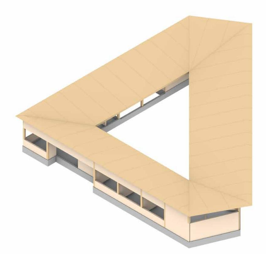
A repetitive structural grid provides the potential to fabricate exterior and interior walls off-site in addition to the structure.
