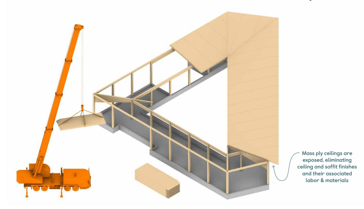
Mass Ply Columns & Beams erect quickly like an assembled kit of parts, minimizing the construction timeline.
