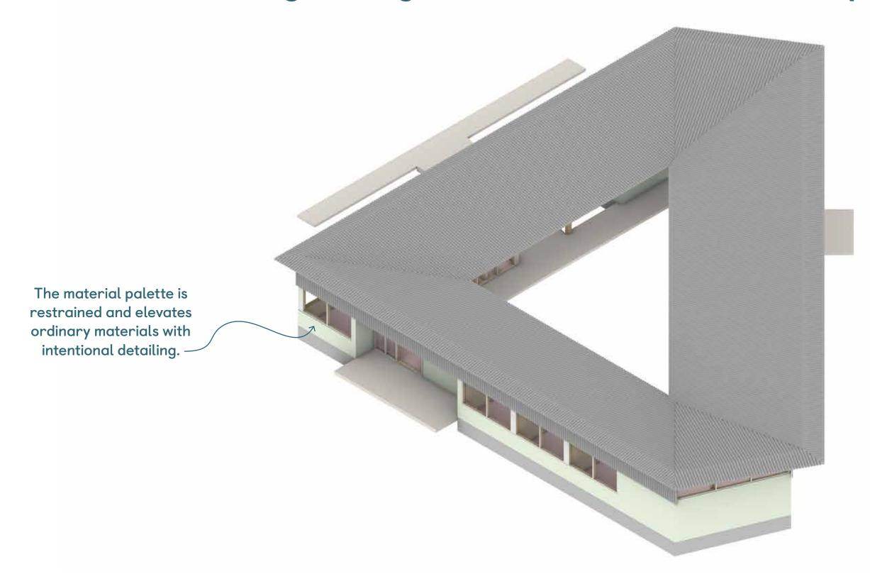
Fiber cement roof & cladding can be installed by framing contractors, reducing specialized labor and minimizing the amount of different trades onsite.
